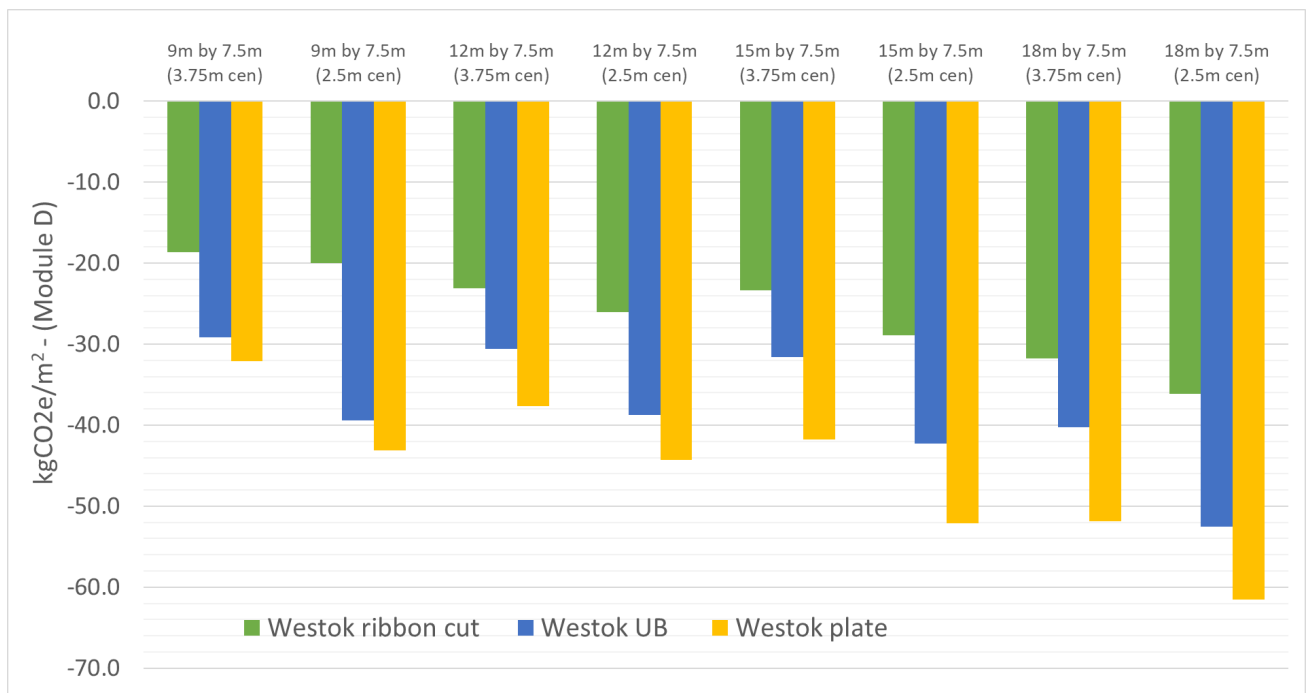
Figure 8 Embodied carbon kgCO_2e/m^2 for module D ( Q_k = 2.5 + 1kN/m^2 ) (Reported as negative to highlight benefit beyond the system boundary)
